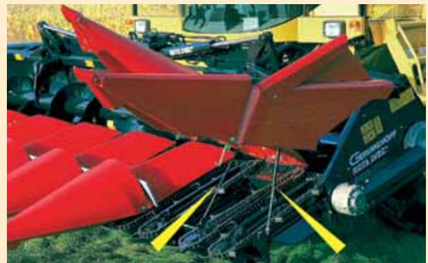
Enhanced protection: Industrial gas springs secure heavy hoods
